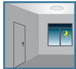
After stand-by period, the sensor switches off the lamp if no motion is detected in its detection zone.
