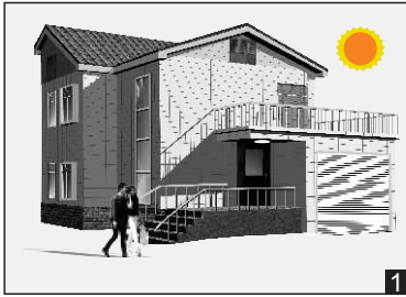
With sufficient ambient light, the sensor does not switch on the lamp.
